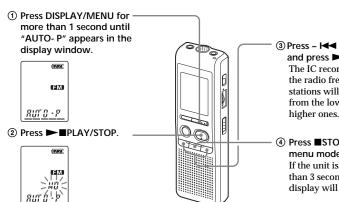
③ Press – I◀◀ or ▶►I+ to select "YES" 🛕 🐷 and press ►■PLAY/STOP. The IC recorder automatically scans the radio frequencies and the stations will be stored in memory
